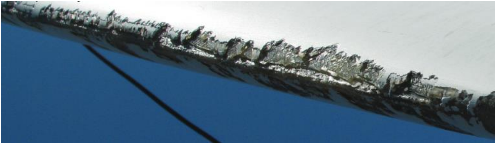
Rempel, L. Rotor blade leading edge erosion-real life experiences. Wind Syst. Mag. 2012, 11, 22–24.
